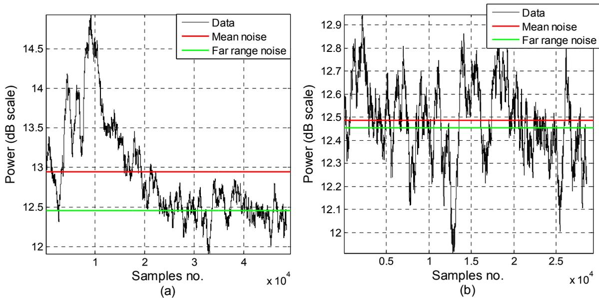
FIG. 3. (a) Power of range bins after the first iteration of the fourth step of the algorithm. (b) Power of range bins after the second iteration of the fourth step of the algorithm.
