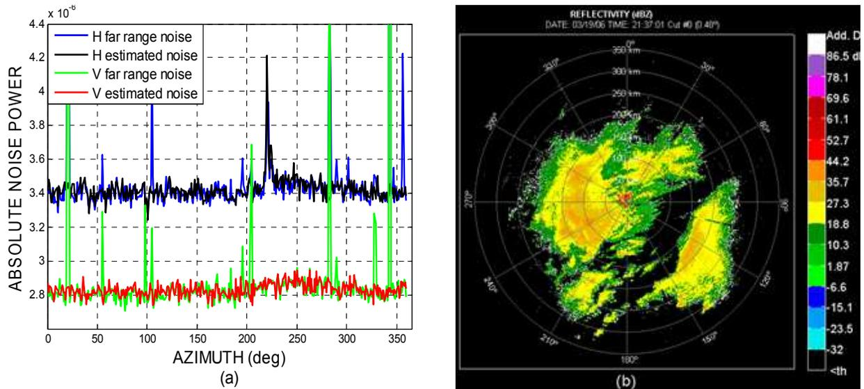
FIG. 5. (a) Noise estimates compared to the far range noise. (b) Reflectivity field with additional detections, resulting from the use of the noise estimation algorithm, highlighted in white.
