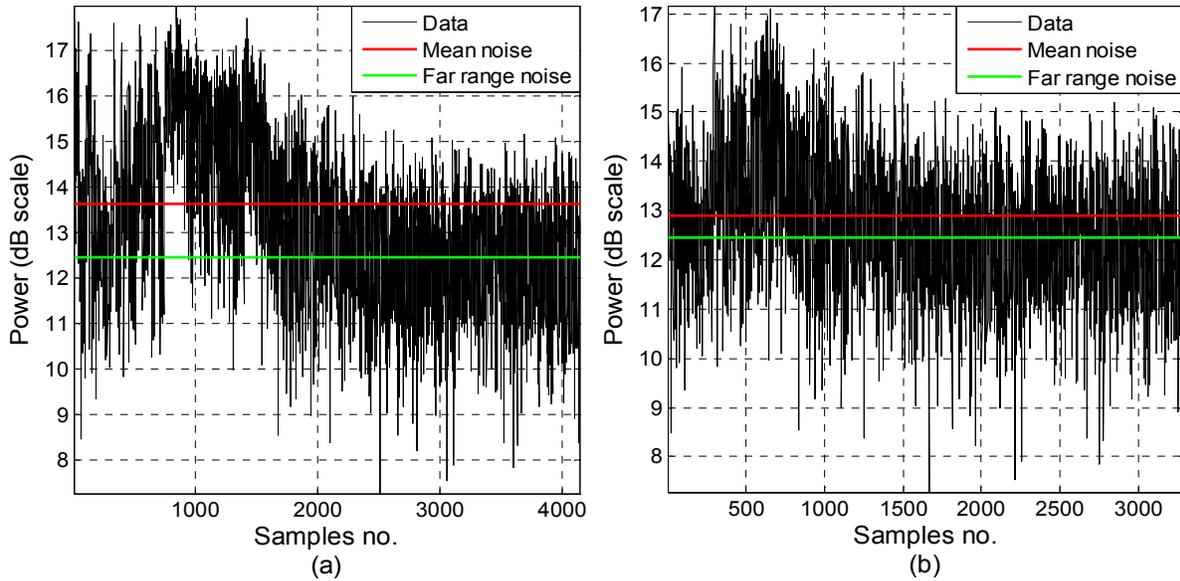
FIG. 2 (a) Power of range bins after the first two steps of the algorithm. (b) Power of range bins after the third step of the algorithm.
