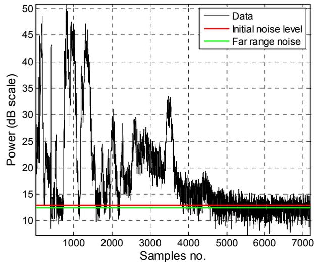
**FIG. 1** Received power as a function of range at the elevation angle of 0.5 deg. The number of samples at each range position is 15 and the range sample spacing is 60 m. The initial and “true” noise values are indicated with a red and green line, respectively. This data was collected using the NWRT PAR in Norman, OK.
