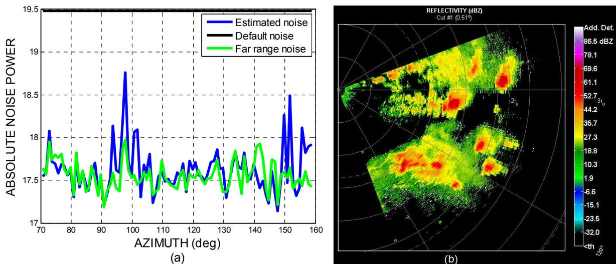
FIG. 4. (a) Noise estimates compared to the initial (default) and the far range ("true") noise, and (b) reflectivity field with additional detections obtained using estimated noise highlighted in white.
