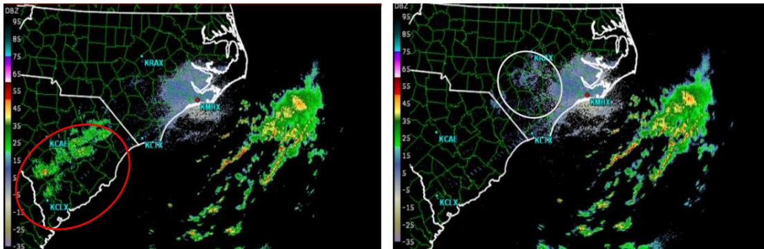
*Radar reflectivity images from the KMHX radar in Newport/Morehead, NC. The current operational processing (left panel) is compared to the proposed processing (right panel). The proposed processing using novel techniques developed by the ART team is more effective at removing ground clutter contamination (red oval) and preserving weak weather echoes (yellow oval).*
