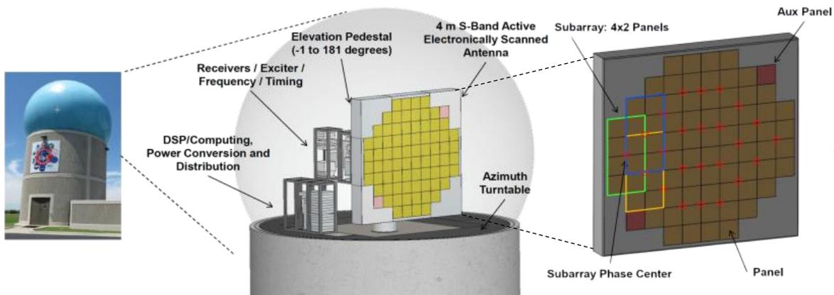
*The ATD is a proof-of-concept system to demonstrate improved capabilities and refine the cost-driving requirements of a multifunction phased array radar (MPAR). It is an S-band, mid-scale, dual-polarized, multifunction, active, electronically scanned PAR at the National Weather Radar Testbed (NWRT) in Norman, OK. It is expected to be operational in 2020.*
