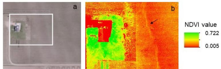
*Fig. 3: UAS-based (a) visible and (b) multispectral imagery for the 12 June 2017 Carpenter, Wyoming, tornado. The outer edge scour of the tornado (black arrow) and damage to freshly laid sod (yellow hues) are shown in (b). These damage indicators are not detectable in visible imagery in (a). Figure provided by Dr. Melissa Wagner.*
